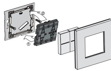
Vertically **EXTENDING** a switch in an existing installation to a dual switch is possible by using a dual vertical cover plate with a 71mm centre distance.
