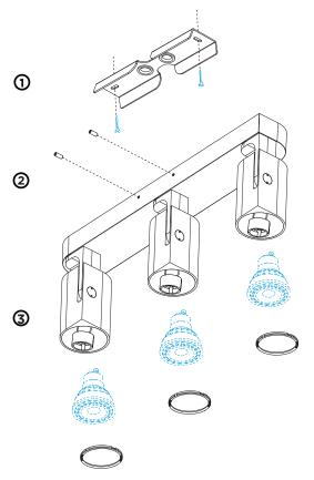
If the installation conditions allow, in order to have a better appearance, we suggest that the side including two allen screws is facing backwards.
