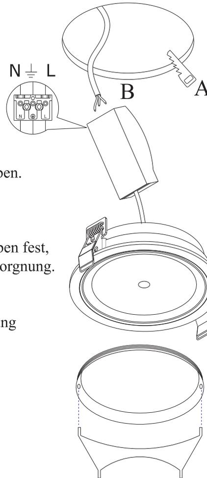
OPTIC IN 1 / HOLE SIZE : Ø94, H50mm
