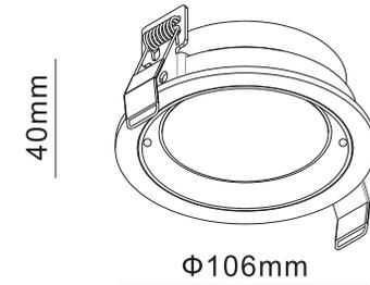
OPTIC IN 1+ / HOLE SIZE : Ø124, H50mm
