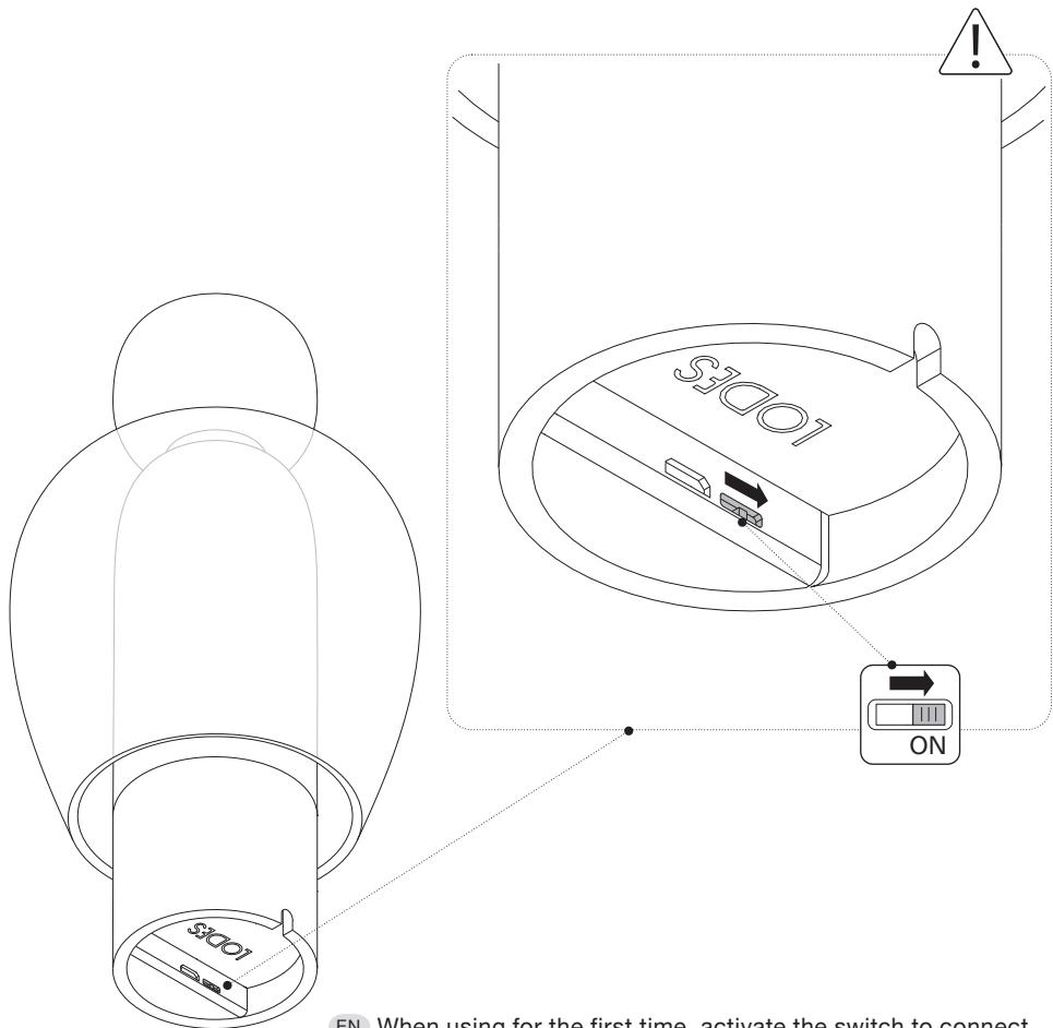
EN When using for the first time, activate the switch to connect the battery.
