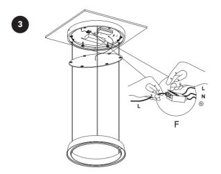
**F:** Connect the cables from both the lamp and the mains power into the terminal as illustrated above.
