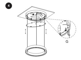
G: To adjust the cable height, push the metal cable adjuster and either pull or feed the cable to the desired length. Release the cable adjuster to secure the cable.
