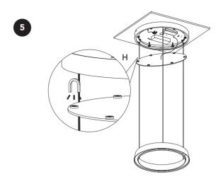
**H:** Mount the decorative ceiling base cover with the magnet fixing points illustrated.
