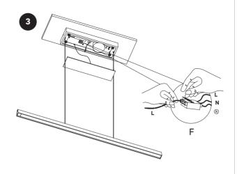
**F:** Connect the cables from both the lamp and the mains power into the terminal as illustrated above.
