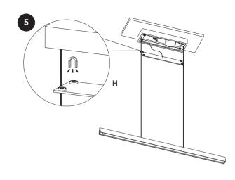
**H:** Mount the decorative ceiling base cover with the magnet fixing points illustrated.
