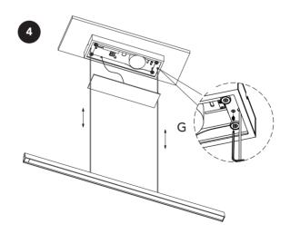
G: To adjust the cable height, push the metal cable adjuster and either pull or feed the cable to the desired length. Release the cable adjuster to secure the cable.
