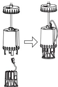
\* For this product, the cable with a plug that comes with the LED module is not needed. Please remove it first and then use the LED module.
