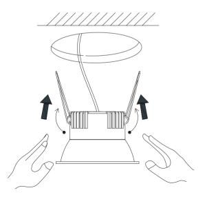
Pull the spring clips upwards and position the lamp into the hole. Slowly release the clips as the downlight is securely positioned.
