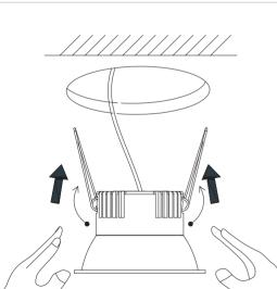
C: Pull the spring clips upwards and position the lamp into the hole. Slowly release the clips as the downlight is securely positioned.
