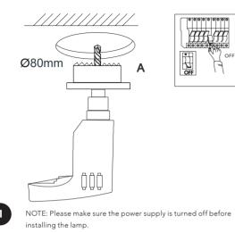
A: Drill an Ø80mm hole at the desired mounting position.
