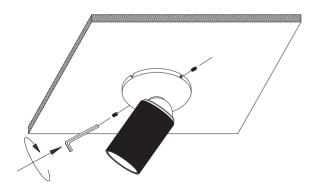
Screw the lamp to the mounting plate as illustrated above.
