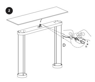
D Connect the power cord and the input line of the lamp body into the terminal according to the identification to fix it
