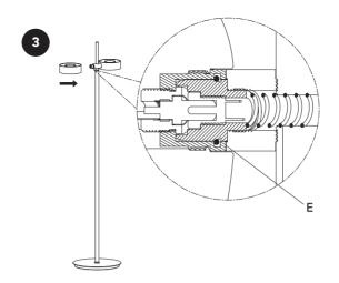
C: Firmly push and fasten the two lamp heads into the pole using the integrated jack system.
