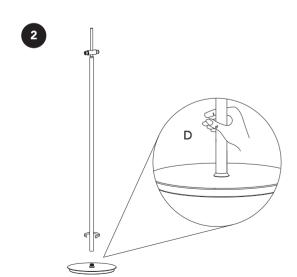
B: Screw the pole into the floor base until you reach a tight fit.
