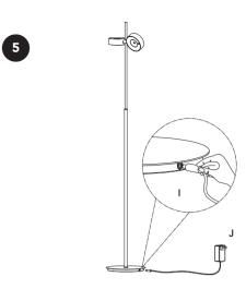
**E:** Plug the DC adaptor to the lamp base, and into the mains power.
