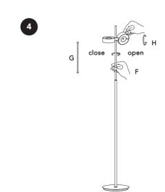
D: The pole height can be adjusted using the integrated "Twist lock" function as illustrated able. Clockwise to fasten, and anti-clockwise to loosen. NOTE: Be gentle when adjusting the pole height to avoid the lamp heads from dropping off.
