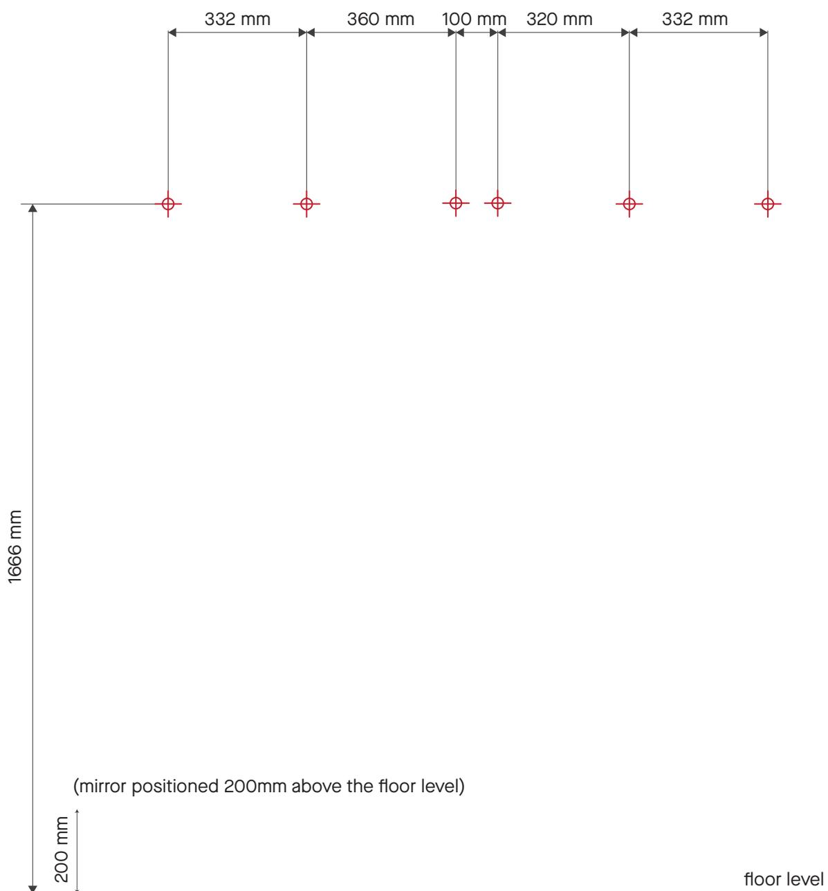
place the mirrors on the washers in the 'open' position
