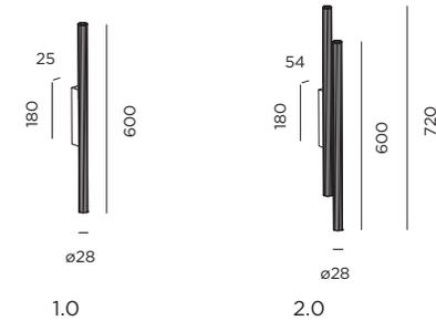
**1** Remove the mounting base from the luminaire by loosening the side socket screw and mount it on the wall with screws (screws are not included).
